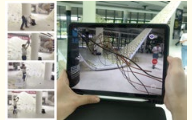
Figure 2 — Student (left) defines a surface by recording spatial positions using a tablet, while another student (right) sees the generated woven structure directly on site concurrently. Photograph: Ye Huzheng, Matthew Tan and Song Qiuji
