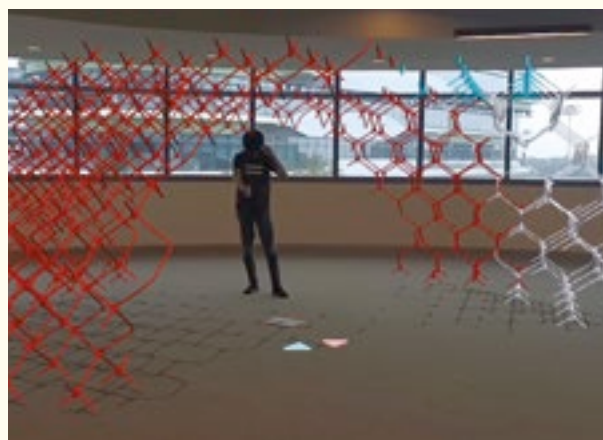
Figure 5 — Student tests the AR app and checks how the hologram is positioned in the space prior to assembly Photograph: Song Qiuji
